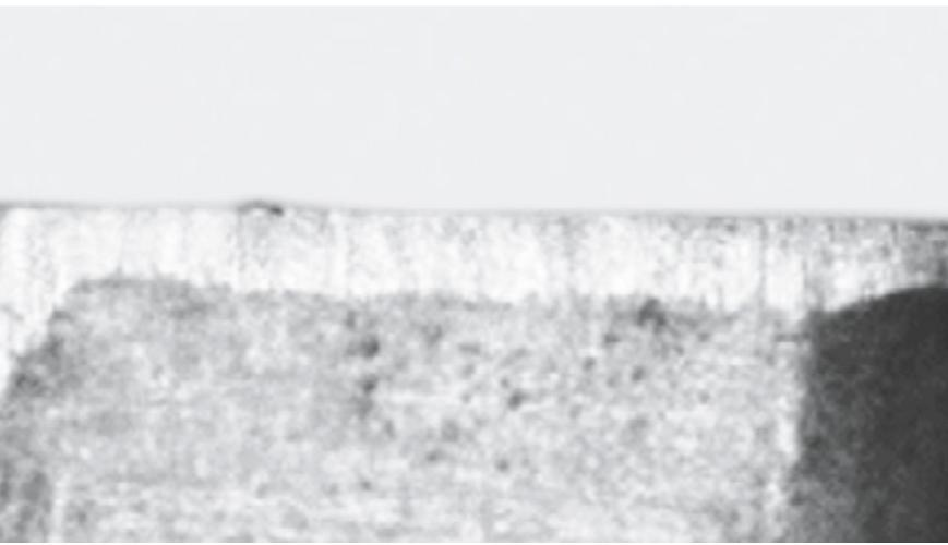
*In high-capacity cutting of SwissCut® SC37Pb, the indexable insert made of carbide exhibits much less wear than when used during the machining of conventional free-machining steel 11SMnPb37.*
